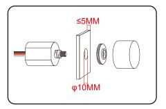
Disassemble the controller and pass through the board in the ways shown above, use a rotating nut to fix the controller, and then press the adjusting knob onto the controller metal rod.
