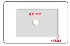
Drill a 10mm diameter hole in advance on the board that requires to install the controller, and the thickness of the board cannot exceed 5mm.
